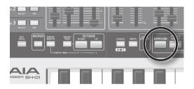
Press the [ARPEGGIO] button so it's lit; the arpeggiator will be on.
