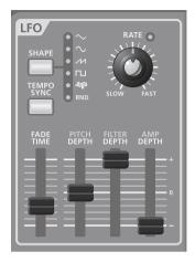
LFO stands for Low-Frequency Oscillator. This is an oscillator with a very low frequency. It can output several different waveforms, including sine wave, triangle wave, square wave, and sawtooth wave.
