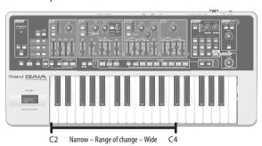
While holding down the OCTAVE [UP/+] button, press a key (C2-C4).
