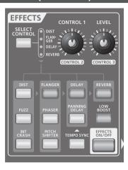
"Effects" allow you to modify or enhance the sound in various ways, such as by adding reverberation or delaying the sound.
